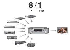
This unit is equipped with 8 HDMI inputs and 1 HDMI output enabling connection to various HDMI compatible devices such as Blu-ray Disc players, game consoles and HD video camcorders.
