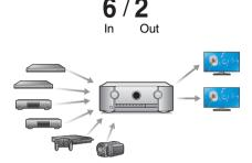
This unit is equipped with 6 HDMI inputs and 2 HDMI outputs enabling connection to various HDMI compatible devices such as Blu-ray Disc players, game consoles and HD video camcorders. This unit is equipped with 2 monitor outputs, enabling you to project the same image at the same time using this unit.
