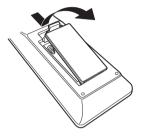
2 Insert two batteries correctly into the battery compartment as indicated.
