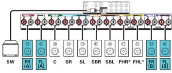
\* The height speakers, ceiling speakers and Dolby Atmos Enabled speakers can be connected to the HEIGHT1 speaker terminals. Set the speaker to be connected from "Height" - "Layout" in the menu. (1287 p. 216)
