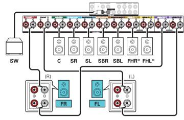
\* The height speakers, ceiling speakers and Dolby Atmos Enabled speakers can be connected to the HEIGHT1 speaker terminals. Set the speaker to be connected from "Height" - "Layout" in the menu. (Pp p. 216)
