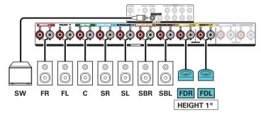
\* The surround Dolby or back Dolby speakers can be connected instead of the front Dolby speakers. In this case, set the Dolby Atmos Enabled speakers to be connected under "Height" - "Layout" in the menu. (12) p. 216)
