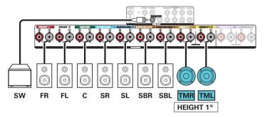
\* The top front or top rear speakers can be connected instead of the top middle speakers. In this case, set the ceiling speakers to be connected under "Height" - "Layout" in the menu. ( pp. 216)
