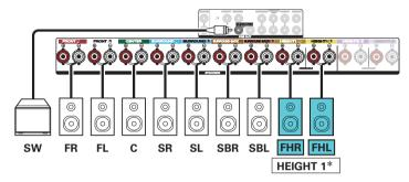
\* The rear height speakers can be connected instead of the front height speakers. In this case, set the height speakers to be connected under "Height" - "Layout" in the menu. (1287 p. 216)
