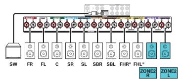
\* The height speakers, ceiling speakers and Dolby Atmos Enabled speakers can be connected to the HEIGHT1 speaker terminals. Set the speaker to be connected from "Height" - "Layout" in the menu. (127 p. 216)
