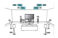
Set "Height" - "Height Sp" to "4ch" in the menu when connecting in this configuration. (<u>Pp. 208</u>)
