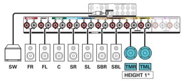
\* The top front or top rear speakers can be connected instead of the top middle speakers. In this case, set the ceiling speakers to be connected under "Height" -"Layout" in the menu. (IPP p. 209)
