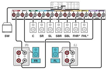
\* The height speakers, ceiling speakers and Dolby Atmos Enabled speakers can be connected to the HEIGHT1 speaker terminals. Set the speaker to be connected from "Height" - "Layout" in the menu. ((Pp. 209)
