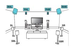
• Set "Height" - "Height Sp" to "4ch" in the menu when connecting in this configuration. (129 p. 208)
