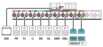
\* The surround Dolby or back Dolby speakers can be connected instead of the front Dolby speakers. In this case, set the Dolby Atmos Enabled speakers to be connected under "Height" - "Layout" in the menu. (127 p. 209)
