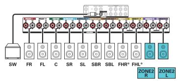
\* The height speakers, ceiling speakers and Dolby Atmos Enabled speakers can be connected to the HEIGHT1 speaker terminals. Set the speaker to be connected from "Height" - "Layout" in the menu. (() 100 p. 209)
