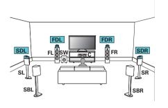
• Set "Height" - "Dolby Sp" to "4ch" in the menu when connecting in this configuration. (127 p. 208)
