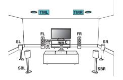
• Set "Height" - "Height Sp" to "2ch" in the menu when connecting in this configuration. (127 p. 208)
