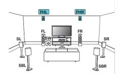
Set "Height" - "Height Sp" to "2ch" in the menu when connecting in this configuration. (<u>Pp. 208</u>)
