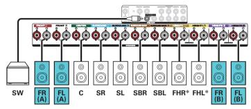
\* The height speakers, ceiling speakers and Dolby Atmos Enabled speakers can be connected to the HEIGHT1 speaker terminals. Set the speaker to be connected from "Height" - "Layout" in the menu. ((Pp. 209)
