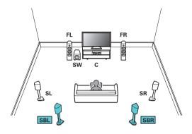
• Set "Floor" - "Layout" to "5ch & SB" in the menu when connecting in this configuration. (12) p. 207)
