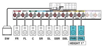
\* The rear height speakers can be connected instead of the front height speakers. In this case, set the height speakers to be connected under "Height" - "Layout" in the menu. (127 p. 209)
