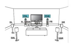
• Set "Height" - "Dolby Sp" to "2ch" in the menu when connecting in this configuration. (127 p. 208)
